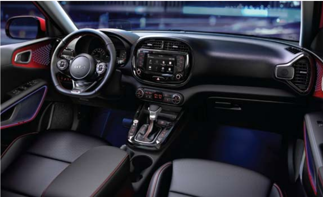
D-cut steering wheel The steering wheel is flat across the bottom for easier driver entry while also adding a racing-inspired touch to the driver's space.
