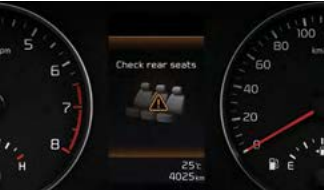
Rear Occupant Alert Don't leave anyone in the rear seats when you park. Rear Occupant Alert tracks door-latch use, and reminds you with a message in the cluster.
