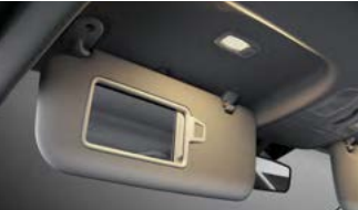
Sunvisor illumination lamps The bulb lamp above the vanity mirror on the driver-side sunvisor lights up to help you see yourself better in the mirror.
